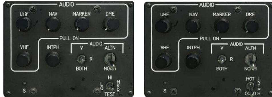
Each audio control panel is equipped with a toggle switch (V, R, and BOTH) to allow for the selection of voice only, recognition or Morse code only, or both voice and recognition channels for the VHF NAV radio. Additionally, there is a toggle switch (ALTN and NORM), which allows for the selection of raw audio if the amplifier stops working.
