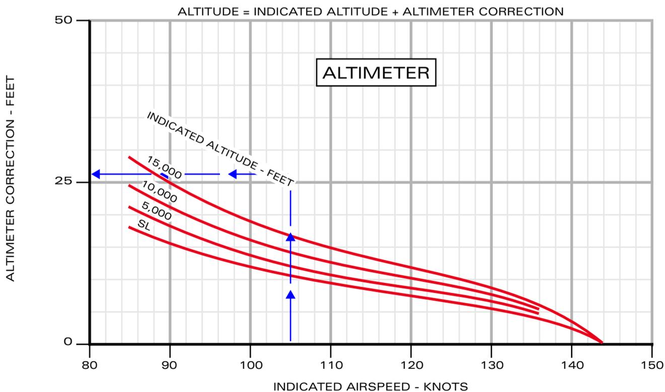
Airspeed/Altimeter Position Correction/Ship - Flaps LDG
