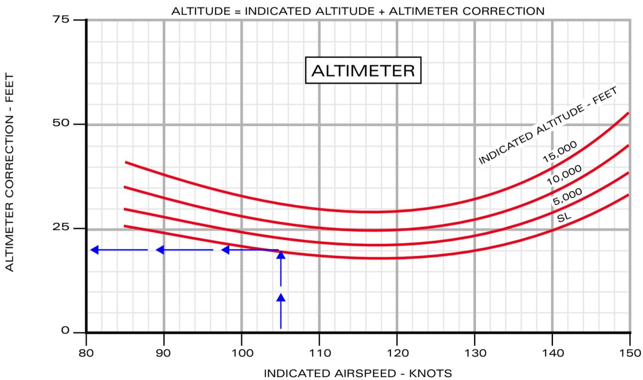
Airspeed/Altimeter Position Correction/Ship - Flaps TO
