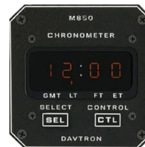
The clock face has a select button (SEL), and a control button (CTL). The digital clock is powered via hot battery bus. Each press of the SEL button will scroll through the available clock functions. Pressing the CTL button will start and reset elapsed time (ET), and is used to set time for GMT, LT, and ET count up and ET count down.
