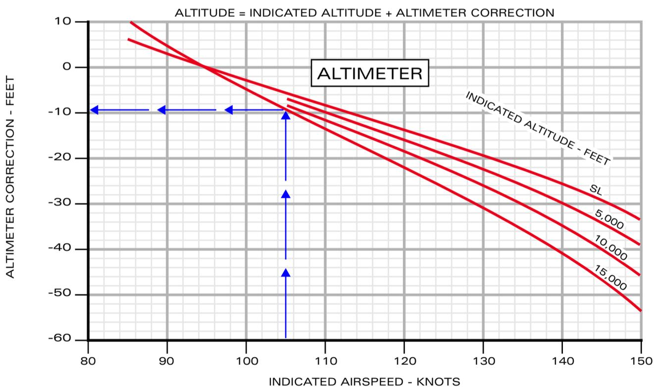
Airspeed/Altimeter Position Correction/Stby - Flaps LDG
