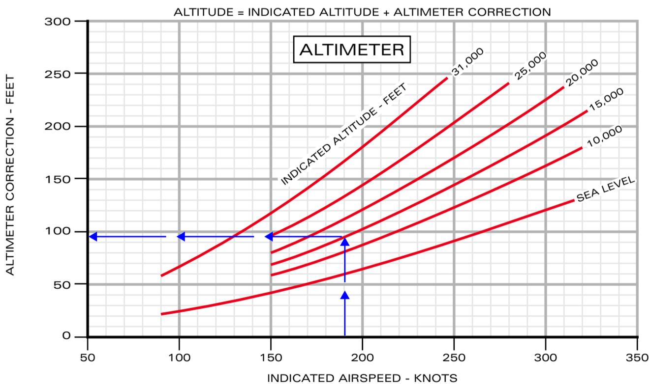
Airspeed/Altimeter Position Correction/Ship - Flaps UP
