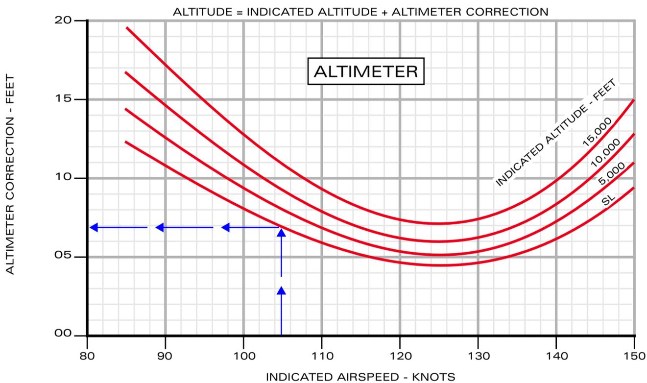
Airspeed/Altimeter Position Correction/Stby - Flaps UP
