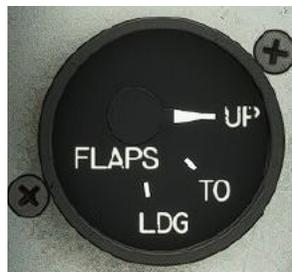
The landing gear control handle in each cockpit has a flap indicator located above it on the lower left side of the instrument panel. The pointer shows the position of the flaps (UP, TO (takeoff), or LDG (landing)). When the flaps are moving, the pointer will be between the designated markings to show this motion. If the power to the indicator is turned off or there is a battery failure, the pointer will move counterclockwise from the UP position.
