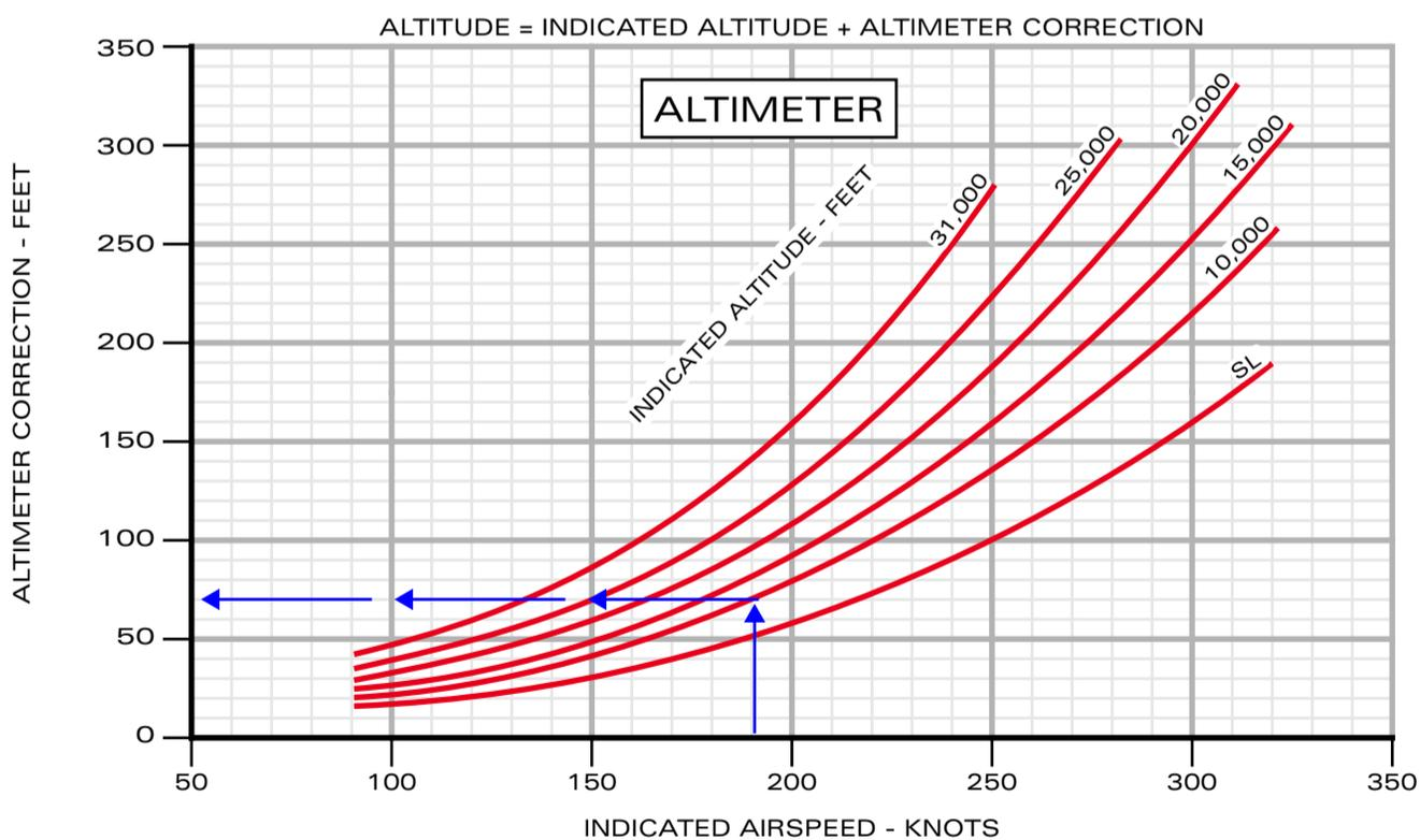
Airspeed/Altimeter Position Correction/Stby - Flaps TO
