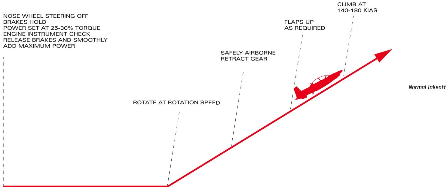
During lineup, it is important to ensure that the brakes are engaged, the nose wheel is centered, and the nose wheel steering is disengaged.
